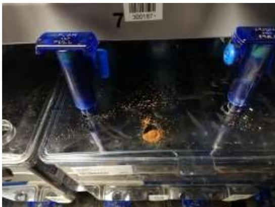
Figure 12- Feed being deposited with wrong nozzle position.
