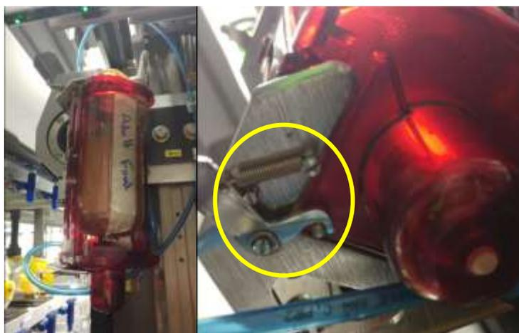
Figure 14- Food bottle in gripper and close-up of spring clamp that holds bottle in the gripper
