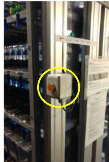
Figure 2- Orange button for calling and/or putting the triton on hold
