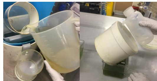
Figure 4- Straining of remaining water (left) before rinsing the strainer into the prepared tank (Right)
